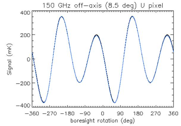
Provides polarization orientation to ~ 0.7 deg accuracy
