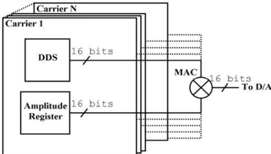
**Fig. 2: The Digital Multi-Frequency Synthesizer algorithm is shown schematically.**
