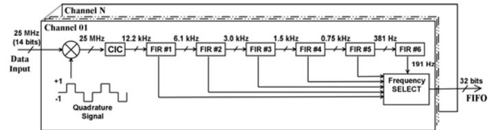
**Fig. 3: The Digital Multi-Frequency Demodulator algorithm is shown schematically.**
