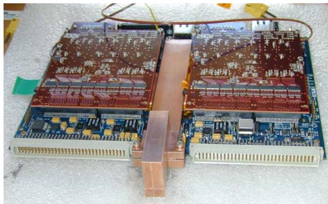
**Fig. 4: The digital fMUX backend electronics. An FPGA motherboard is shown (large lower blue board) with two of its analog converter mezzanine boards attached (smaller upper red boards) and the copper convective heat pipe and conductive heat sink.**
