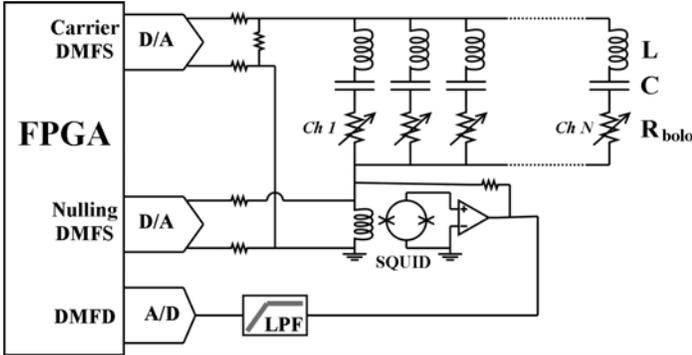
**Fig. 1: The digital frequency domain multiplexer system is shown schematically.**
