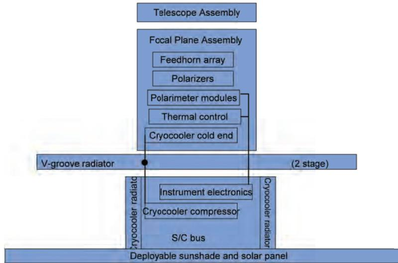
**Figure 2.** Block diagram of PILOT. The V-groove radiators provide excellent isolation of the warm and cold parts of the system, intercepting conducted heat from spacecraft bus and radiating it into space, as well as providing efficient precooling at  $< 50$  K for the cryocooler.
