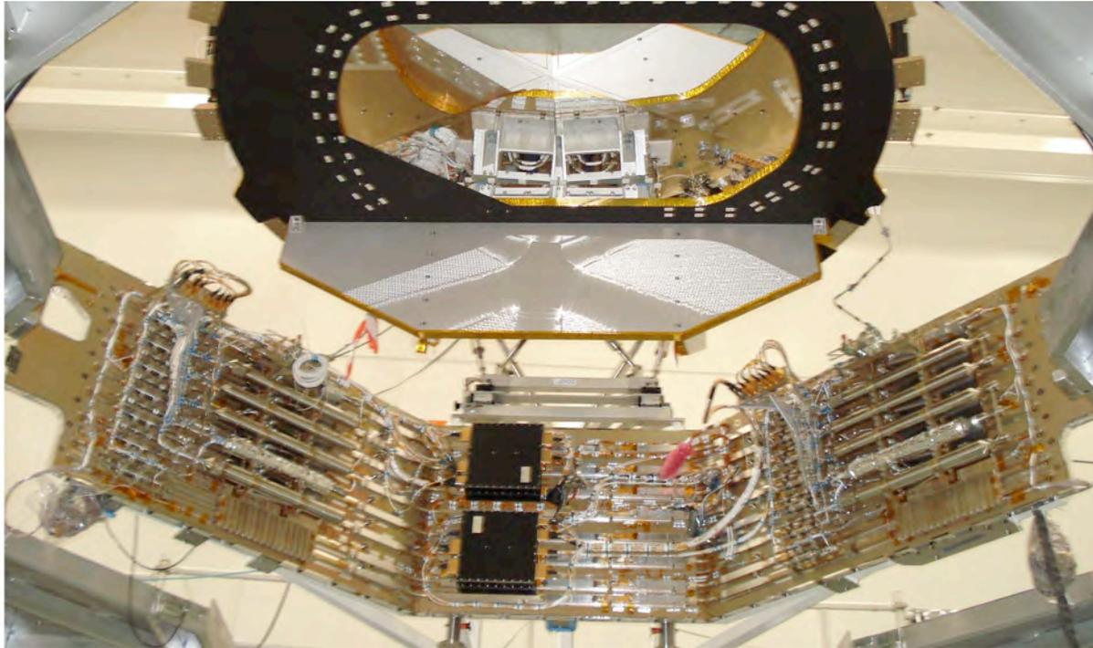
**Figure 5.** The 20-K hydrogen sorption cooler for Planck. Reconfigured to supply a single JT expansion valve, appropriately sized for a 45 K precool temperature, the Planck cooler would provide over 4 W of heat lift at 20 K. It therefore provides a high TRL existence proof for the viability of cooling a large array of amplifiers in space.
