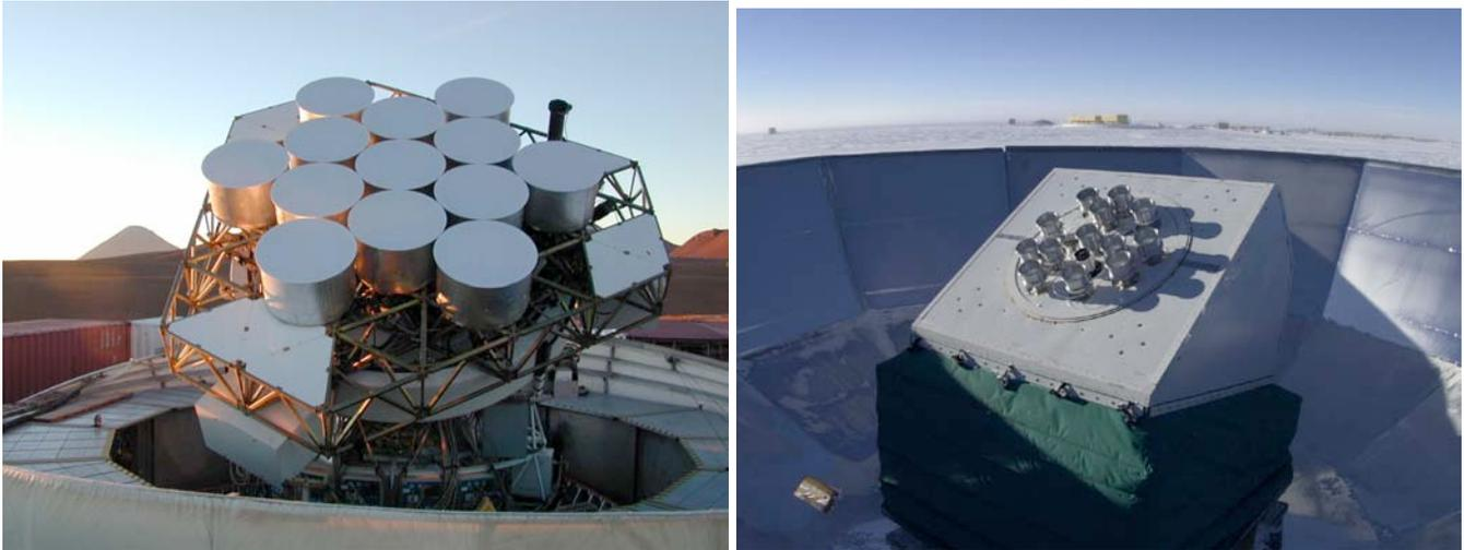
**Figure 8.1:** *Left: the CBI CMB interferometer in the Atacama desert in Chile. Right: the DASI CMB interferometer at the South Pole. An interferometer forms effective beams by correlating signals between the many antennas.*
