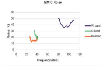
Figure 6: noise curves of one of our MMIC amplifiers. Two dozen of the 90 GHz amplifiers are currently operating in CAPMAP with a typical receiver noise of 50 K. The 40 GHz amplifiers have 20 K typical noise and are also operating in CAPMAP. We have demonstrated similar band-average performance in the QUIET modules.
